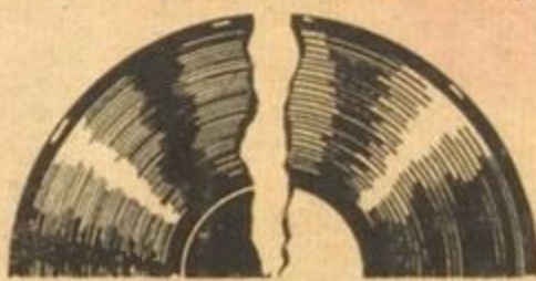
New Improved Record (Closer Grooved) vs Old Style Record (Grooved Too Far Apart)
